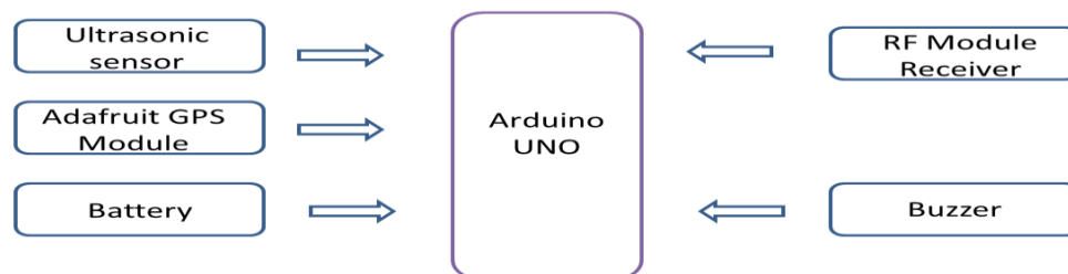
Fig. 2.1 Block Diagram for smart blind stick
